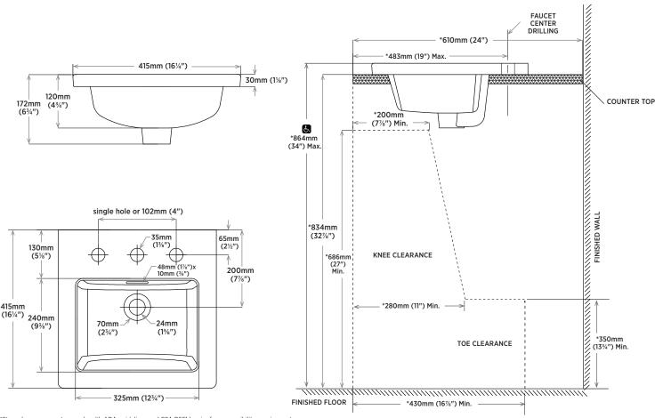
NOTE: \*Starred measurements comply with ADA guidelines and CSA B651 barrier free accessibility requirements.
