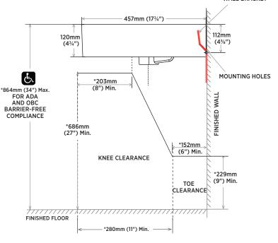
NOTE: \* Starred measurements comply with ADA and OBC barrier free accessibility requirements.
