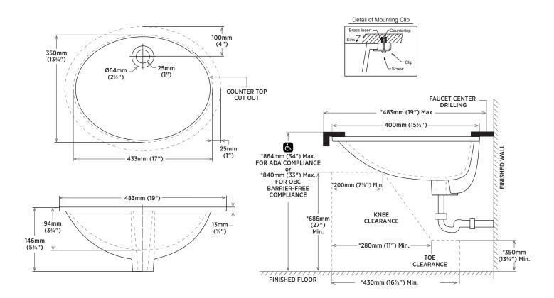
NOTE: \* Starred measurements comply with ADA and OBC barrier free accessibility requirements.
