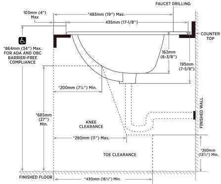
**NOTE:** \* Starred measurements comply with ADA and OBC barrier free accessibility requirements. **\( \D**\) Dimensions shown for location of supplied and waste are suggested.
