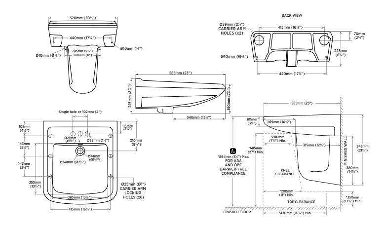
NOTE: \* Starred measurements comply with ADA and OBC barrier free accessibility requirements
