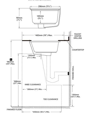
NOTE: \* Starred measurements comply with ADA and OBC barrier free accessibility requirements.
