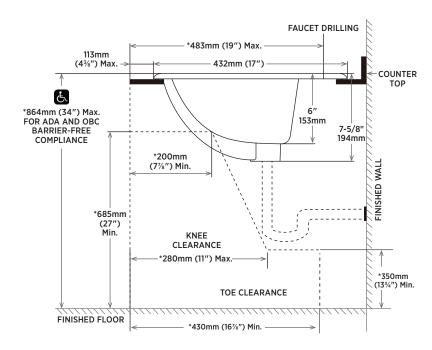
**NOTE:** \* Starred measurements comply with ADA and OBC barrier free accessibility requirements. ▲ Dimensions shown for location of supplied and waste are suggested.
