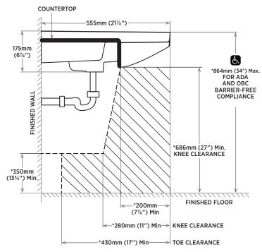
**NOTE:** Starred measurements comply with ADA and OBC barrier free accessibility requirements.
